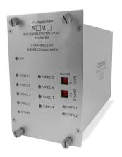
The ComNet<sup>TM</sup> FVT/FVR80D2SFP series optical video link provides transmission of eight 10-bit short-haul quality digital video channels, two bi-directional data channels and one bi-directional contact closure channel through a selectable small form factor pluggable module (SFP). The data channels support RS232, RS422 and 2 wire and 4 wire RS485. Plug-and-play design ensures ease of installation and no electrical or optical adjustments are ever required.
