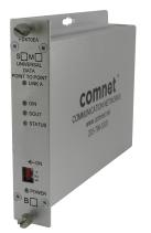
The ComNet<sup>™</sup> FDX70 data transceivers provide point-to-point transmission of simplex or duplex EIA RS232/RS422/RS485 (2W/4W) data signals over one single mode or multimode optical fiber. The transceivers are transparent to data encoding allowing for broad-range compatibility. Models within this series are available for use with multimode or single mode optical fiber. Plug-and-play design ensures ease of installation requiring no electrical or optical adjustments.
