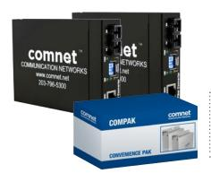
The ComNet™ CWFE2SC(M,S)2 Ethernet media converters are designed to transmit and receive 10/100 Mbps data over multimode or single mode optical fiber. The electrical interface will Auto-Negotiate to a 10 Mbps, or 100 Mbps Ethernet rate without any adjustments. The optical interface operates at a 100 Mbps Ethernet rate. These media converters are commercial grade for light industrial use.
