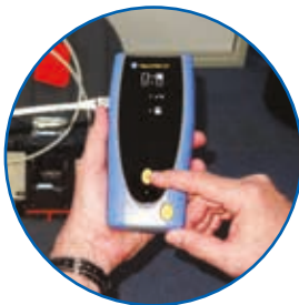
Autotest from remote unit for one person testing
