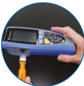
Replaceable RJ45 contacts
